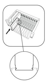
In the case of processing of encrypted TV channels, insert the CAMs and the operator smartcards in the FLOW SEC modules.
