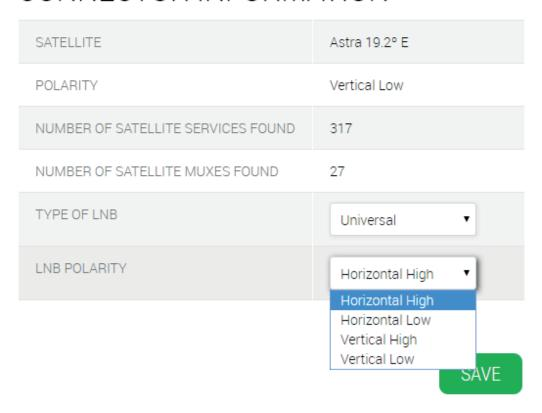
In LNB POLARITY, select the desired polarity, Horizontal High, Horizontal Low, Vertical High or Vertical Low.
