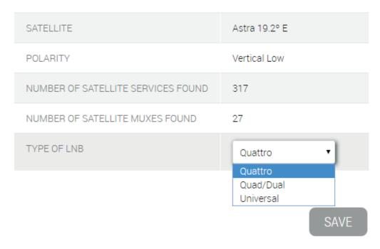
In the case you use a 13/18V without tones switching LNB (tipically used in Australia) select TYPE OF LNB: Quad/Dual.
