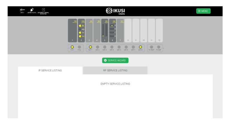
In the example, the top bar informs that two antennas have been connected: one terrestrial antenna identified as DTV1 and one satellite dish pointing to Astra 19.2°E satellite. Also, you could see that RF signal that has not been generated by Ikusi Flow has been detected.
